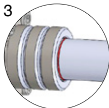
3 With Socket on Drill in low gear, drive down to the red Reference Line
